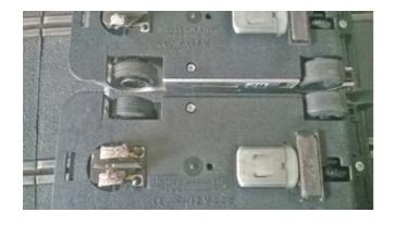
Company obviously took the opportunity of changing the branding to Hornby when altering the wiring arrangement to the slot guide from eyelets to contact strips.
