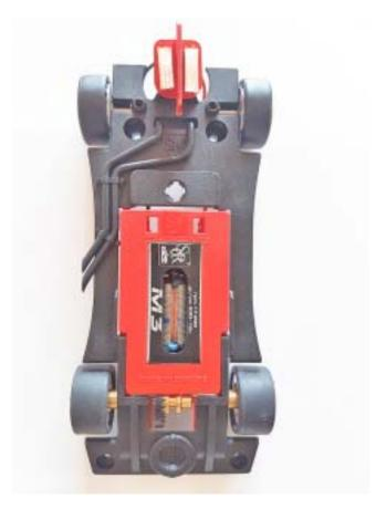
again of high detail but let's look closely at the real change. The layout of the chassis has completely changed, as you can see in the comparison photograph. The CHRONO series is running an in-line motor instead of the older sidewinder-mounted motor. Changing the motor from sidewinder to in-line gives the car a better centre of gravity, in turn making the car a more user-friendly track-ready setup. Since we are talking about the new in-line setup, you will
