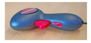
speed-limiting function appears more reliable and less susceptible to ill treatment: the previous screwdriver slot could easily be abused resulting in a damaged mechanism. The handle feels snug and should be just as suitable for smaller hands.
