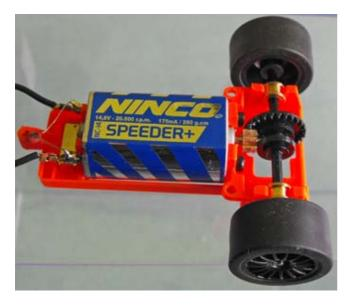
absorb minor undulations in track surface and removes the need for loosening the body from the chassis. The front axle can now be adjusted using small Allen screws to fix its rest height and restrict tilt.
