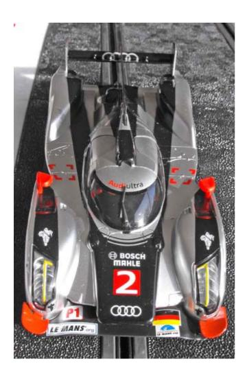
model which differs from the original design is the slight bulge behind the cockpit which is necessary to take the long-can motor beneath the body. This does not at all detract from the sleek look of the car and I imagine will mainly go un-noticed.
