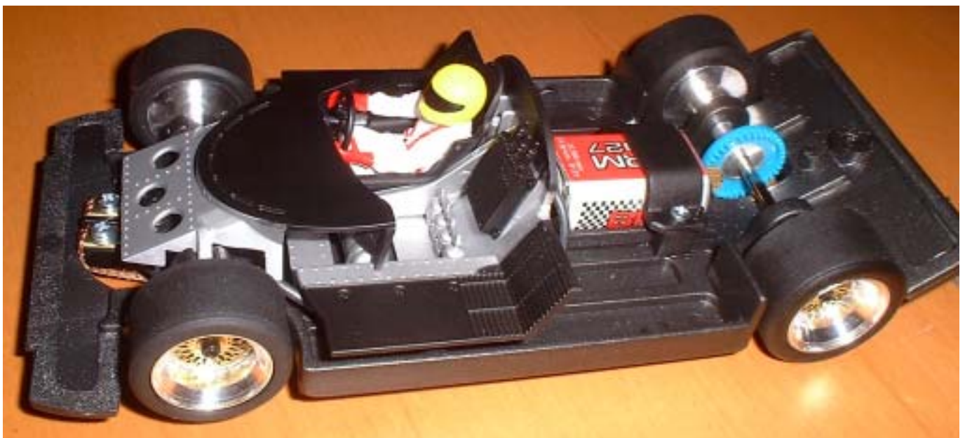
Assembled chassis with additional tube modification to left of the crown gear
