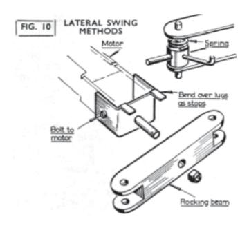
The lateral swing to the axle can be very easily studied in the V.I.P. type of axle, where it
