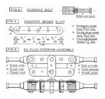
that the three links should all be the same length, and that movement is free without being sloppy, or the car wheels will tend to wobble on the straight, when the car should be travelling its fastest (Fig 7).
