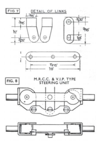
This is particularly suited to cars which have a plate type of chassis, and involves very little more work, indeed it is in some cases a good deal simpler. The stub axle can be made in a variety of forms, possibly the happiest is to drill out a piece of square section brass, drill out the stub axle on the one side, and drill out at right angles, where the square section helps, to make the link, and then right through the centre to take the actual pivot post (Fig. 9.)
