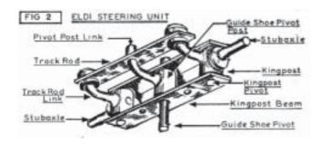
Many people will prefer to make their own units, which can then be built to suit their particular car and scale. Our first unit then is offered to those with the barest minimum of equipment and entails nothing more difficult than drilling a few holes, soldering a joint or two, and wielding a small saw, file or tin snips.
