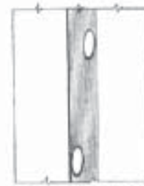
Fig. 4. Original Varcoe steering system for 1/40 scale can be elaborated. Shown with 3/32 in. dia. pins at 3/8 in. centres. Connected to front and rear track links will be flexible, non-jerky and permit minimum radius of track
