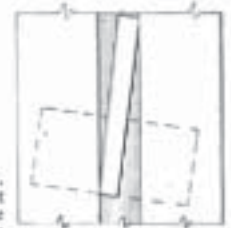
Fig. 2. M.R.R.C. flat plate guide shoe 9/16 in. long by 1/16 in. thick. Shoes such as this must be of non-conducting material as they will normally touch both sides of slot at once. The shoe swings out to its limit and tends to somewhat jerky motion
