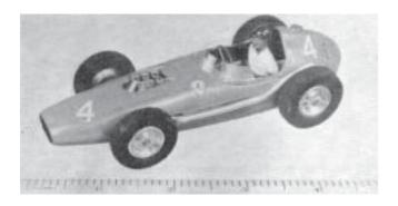
The windscreen and its small brother round the Webers are both made with three lugs each, which fit into razor-thin slits, one on each side of the body, in the case of the windscreen, and one at the front. The edges and lugs of the screen are well covered with Araldite, and then eased into position. Also, in the case of the windscreen, the rear-most edges are firmly Araldited to the sides of the tail, and afterwards covered with Isopon, which is rubbed down to merge with tail when dry.
