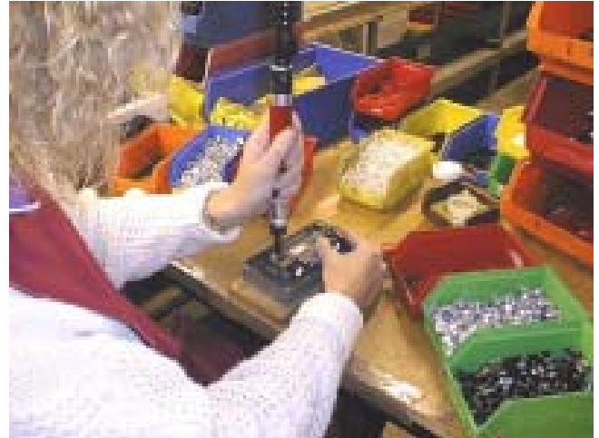
A Megane 'Diac' has its underpan screwed to the body.
