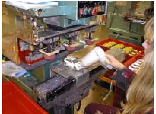
Here, a three-colour 'tampo' machine is used to start the printing on the original Scalextric Toyota Corolla livery.
