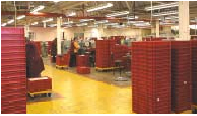
The tampo-printing room is a dust free zone, hence the plastic trays not cardboard boxes.
