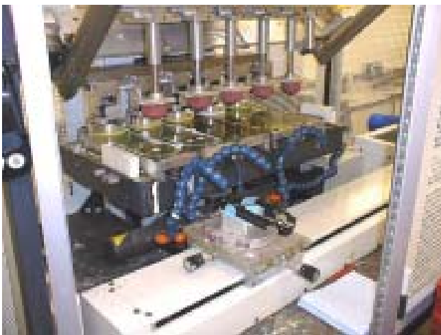
This ink-printing machine is in the process of stamping five different colours on to the black body of the Vauxhall Vectra body.
