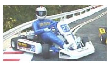
It is obviously that the karts have been designed to run on Ninco track which is wider but I would still recommend borders. Another item that shows that these have been designed from the ground up to run on Ninco track is the placement of the magnets. Yes, magnets, plural. There are two small round magnets fitted just below the fuel tank which align with the power rails in the track. These are slightly further apart than on Scalextric/SCX track, hence my comment.
