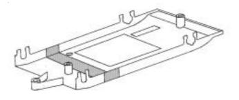
The E-Type is a typically narrow 1960s motor car and to fit the axles to this model you need to reduce the track to 31mm. This involves cutting the axles and also filing a little material off the inside of the wheel hubs so that they clear the bodywork and don't rub on the chassis.
