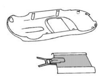
Cut the centre section (shaded grey ) out of the lower body/chassis and glue the remaining sills to the upper body with a strengthening piece of scrap plastic along the inside of the join.
