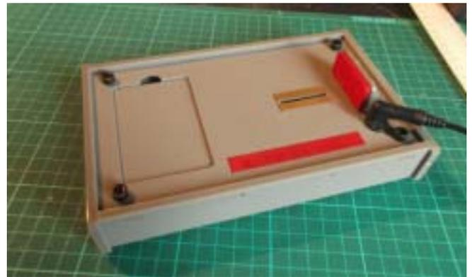
Well firstly is the tyre truer itself, a grey rectangular box with a slot for the guide, stop plate, a power socket for the mains connection (12-16Volt DC) and a recess for the sanding/cleaning sheets. The sanding sheets, eight in total some on a thicker plastic backer, which fits in the recess on the truer and others with self adhesive backing and four sheets for cleaning the tyres, again a couple on plastic backers and two with self adhesive backing to replace the others when worn.
