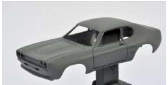
was given a final wipe down with a 'tack cloth' and painted in a dust free environment (or as dust free as any environment can be). Several light coats were applied with 15 to 20 minute intervals in between each application.
