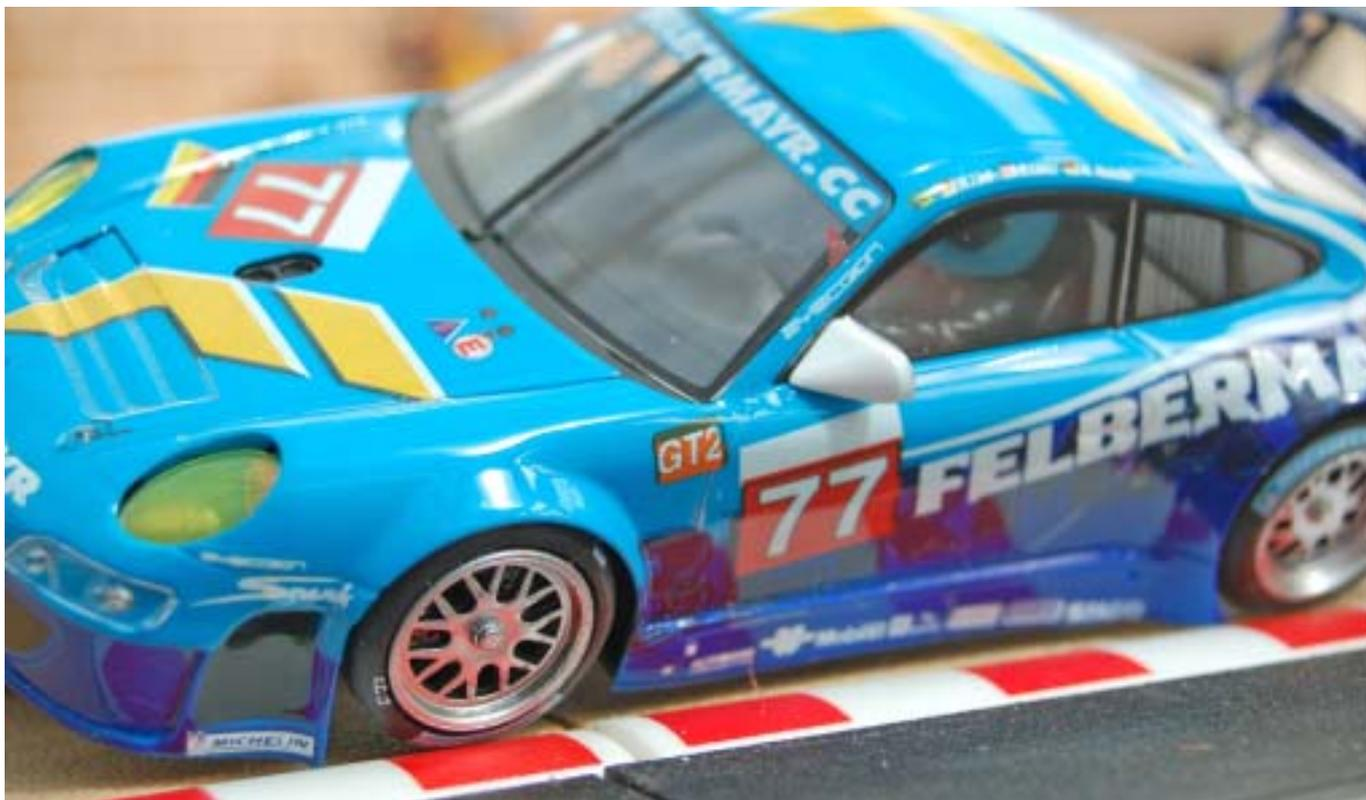
of any damage. With the dual magnets removed, the lead wires relocated and the tyres lightly trued it was a delight! No record breaker but it would certainly be good fun to race with its grippy tyres and fun tail out attitude.
