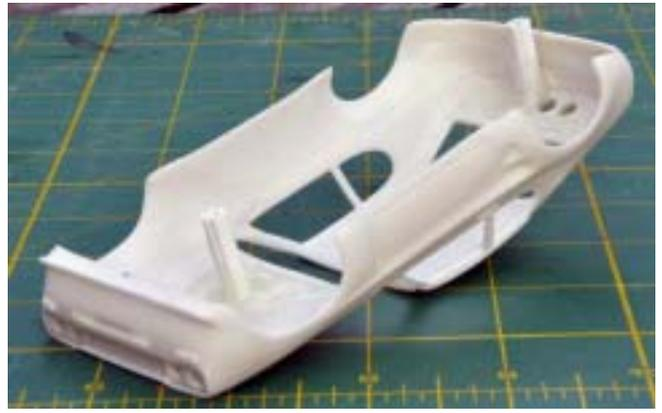
for a day or two to fully cure. The primer will also highlight any imperfections and these can be filled, sanded and additional primer applied.
