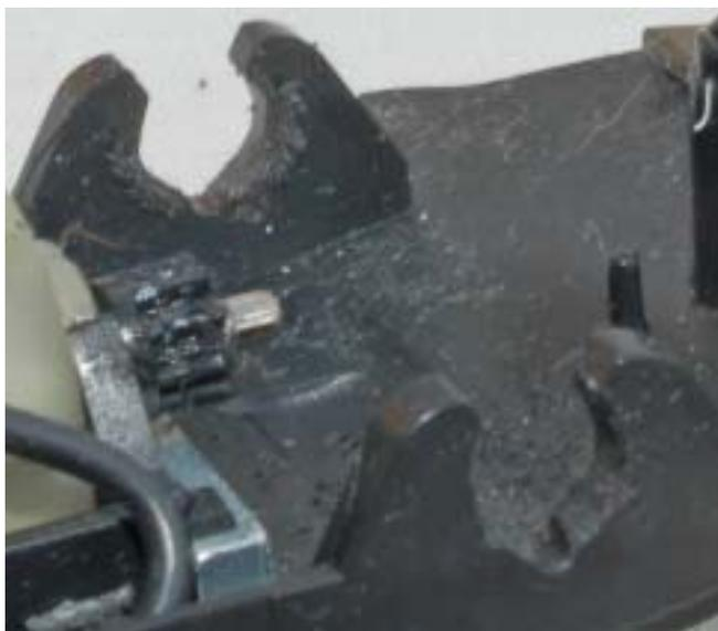
one wheel and another wheel appeared to be cracked around the centre. And, just to underline the poor quality, one headlamp was out of position and the lower edge of one side looked as though it had been caught by a soldering iron.
