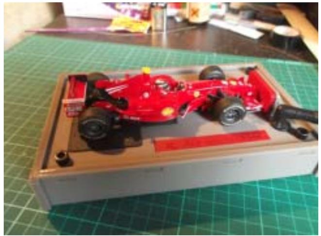
consistent contact with the rear tyres. It could be argued you could get the same result using a piece of sandpaper but I must confess that using the truer, means your car is securely located and you only need one hand rather than having to hold the car in one hand, hold the sand paper in the other and then squeezing the throttle with either your foot or in your mouth!
