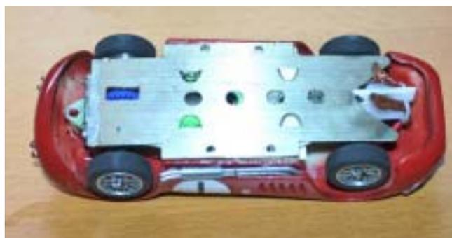
**Underside of the Maserati showing GT Models new handling plate**
