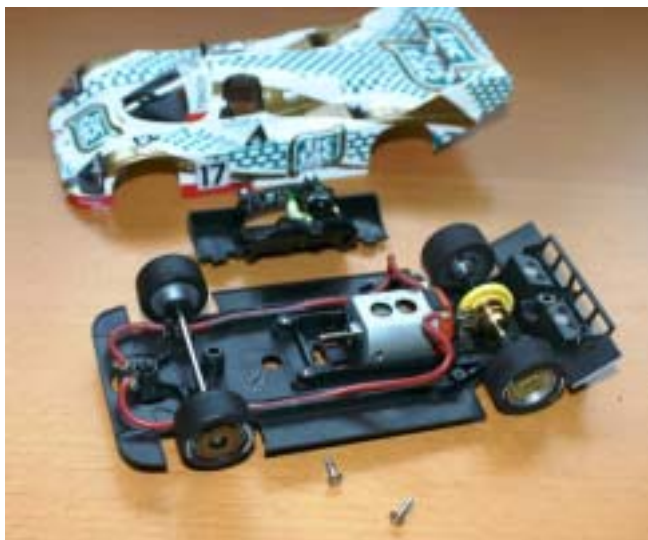
The Cockpit and chassis layout of the new Porsche
