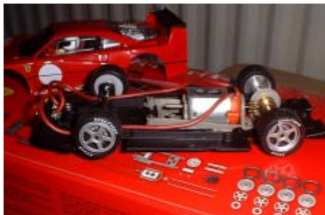
F40 chassis assembled in standard in-line form
