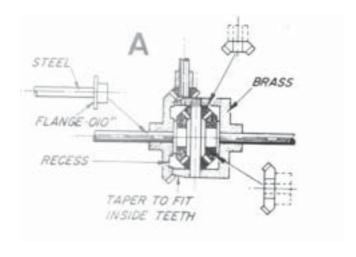
The two 2.5:1 sun wheels had the boss removed. This was achieved by turning off the peened over portion and pressing out the bush
