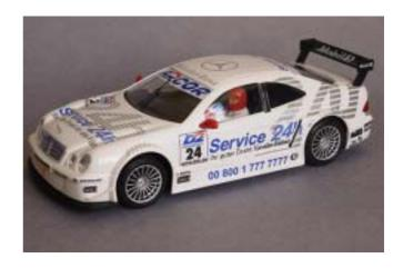
It has very good acceleration and cornering capabilities. The fat slicks, NC2 motor and the centrally mounted magnet provide smooth progressive predictable handling, there is none of that sudden letting go resulting in a high speed barrel roll associated with rear mounted magnets. Ninco have got it right in the great Magnatraction debate – their mid chassis magnet allows feel and control on the throttle rather than taking over and actually doing the whole job for you.
