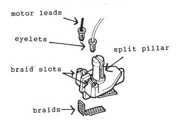
gives electrical continuity to the motor. The pick up guide is connected to the underpan of the car by a split pillar which fits into a collar in a profiled, open D' shape in said underpan allowing the guide to rotate and pivot when the car turns.
